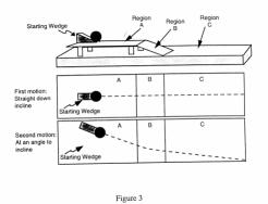
Figure 3.: Apparatus used in the tutorial entitled Changes in Energy and Momentum that helps students learn to apply the work-energy and impulse-Momentum theorems. The ball is released from the same height on the starting wedge in the two cases.
